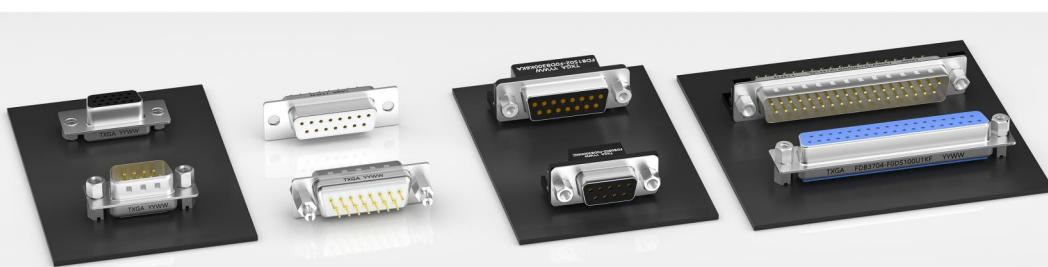
Designed for mixed high-frequency and low-frequency signals, high-current, and high-density device interconnection, D-Sub connectors offer robust and reliable connectivity. Available with push-lock and screw-lock mechanisms for secure mating. Configurations include single-row, dual-row, triple-row, and quad-row options, supporting 1 to 78 positions. Multiple mounting options, through-hole soldering, IDC, crimping, and soldered wire termination.
