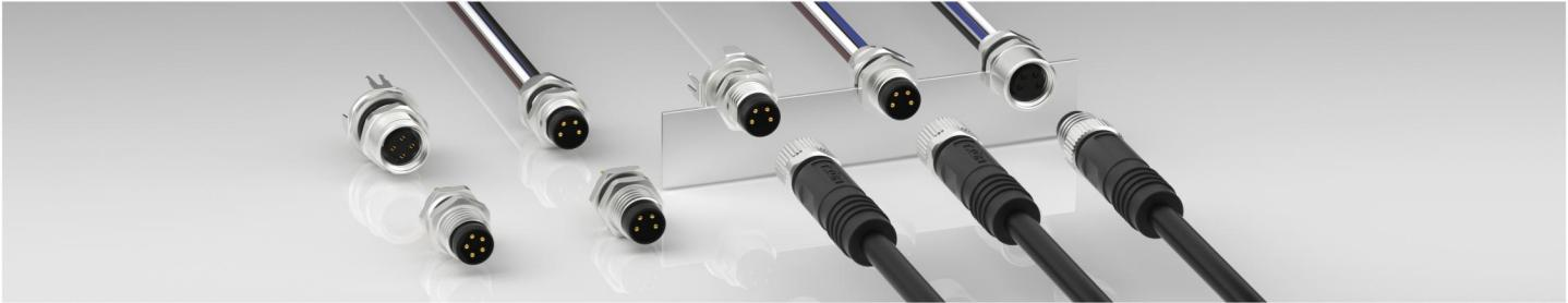
Compliant with IEC 61076-2-104 standards, the M8 circular connectors offer IP65/IP68 protection. Available in shielded and unshielded versions, the shielded models effectively reduce EMI and RFI interference, ensuring stable and reliable signal transmission. With a rated current of 1.5A to 4A and a rated voltage of 30V to 63V, these connectors come in A, B, and D coding options and support through-hole soldering and wire soldering installation methods.
