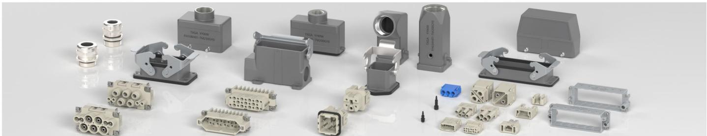
Protection level is IP65, supporting over 500 mating cycles. With a voltage rating of up to 690V and current rating of up to 63A, it ensures excellent electrical contact and low-resistance transmission, supporting high-density circuit connections. Available in 2, 3, 4, 5, 8, 12, 24, 25 and other contact configurations.
