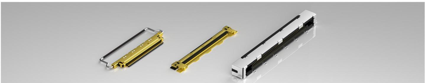
LVDS (Low Voltage Differential Signaling) connectors are designed for high-speed data transmission while saving PCB space. Pitch 0.5mm. Available positions 30pins, 40pins, and 51pins. Current rating 0.5A. Voltage rating 50V to 100V. Mounting options Surface-mount and wire-soldered versions. Ultra-low profile 3.75mm height.
