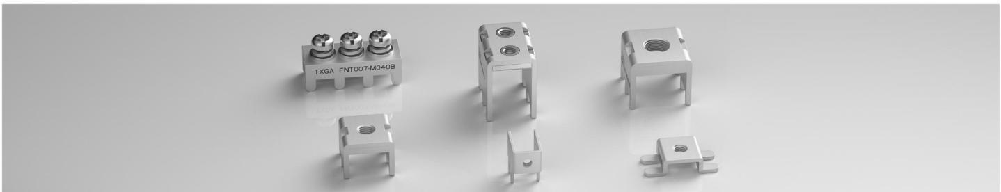
Available in M3, M4, M5, M8 screw sizes with through-hole or surface-mount options. 90°/180° mounting orientations. Current rating 40A-120A. Stainless steel washers provide corrosion resistance and compatibility with square/round head screws.
