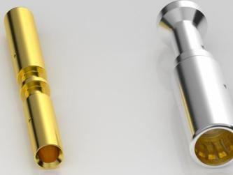
Gold/silver plating with customizable thickness. 4A-200A current rating supports hot-plugging. Internal spring mechanism ensures multi-point contact and low resistance.
