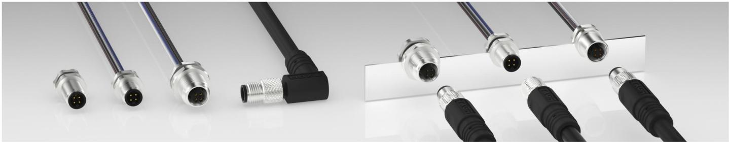
Compliant with IEC 61076-2-105 standards, the M5 circular connectors are available in straight and right-angle cable-mount options. With an external thread diameter of only 5mm, they are ideal for compact device installations. Featuring an IP68 protection rating, they are available in 2, 3, and 4 positions.
