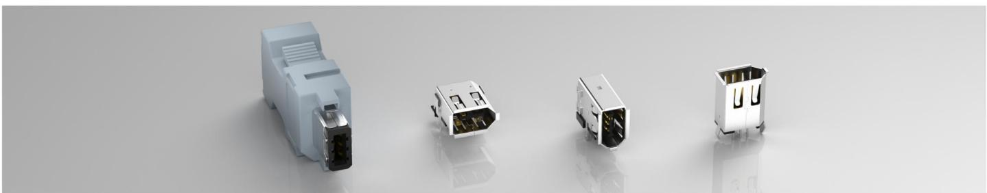
Featuring a six-wire design supporting 400Mbps data transfer and power delivery. 6 positions, 1A-1.5A current rating, 30V-40V voltage rating. UL94 V-0 flame retardant. Hot-plug capable.
