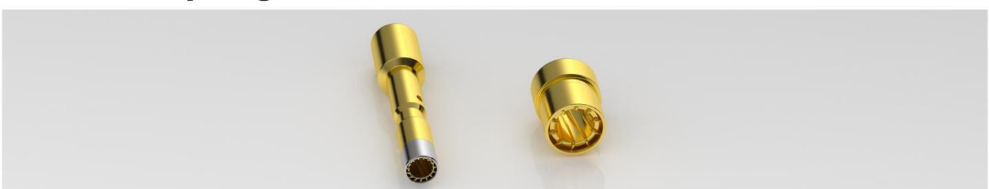
Dual-curved spring design creates multi-point contact for reliable connectivity. Smooth mating cycle suitable for high-frequency applications. 60A current rating, 0.5mΩ contact resistance enables high-precision signal transmission.
