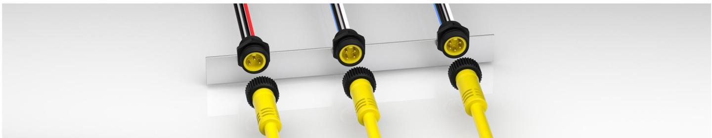
The 7/8" connectors utilize a threaded locking mechanism. The plug features an integrated anti-vibration gasket, which effectively prevents loosening and ensures a secure connection. The cables are constructed with STOOW American-standard power cords, which are resistant to acids, alkalis, UV exposure, oil, and mildew. These connectors are available in 3, 4, and 5 positions.
