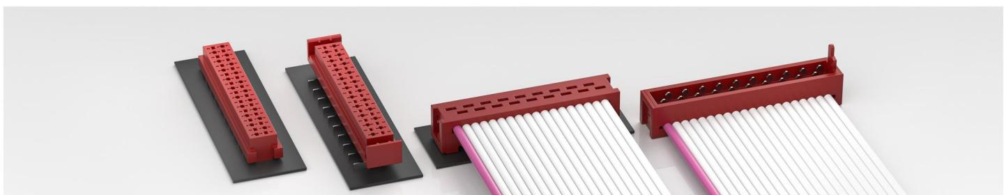
Terminals adopt an elastic structure to absorb environmental vibrations, reducing friction between contacts and pins. Pitch 1.27mm, available in 4, 6, 8, 10, 12, 14, 16, 18, and 20 positions. Flame retardancy UL94 V-0. Available in through-hole soldering, IDC, and surface-mount installation options.
