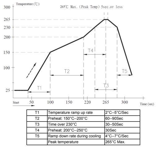
**Note:** Please check the reflow soldering condition by your own devices beforehand. Because the condition changes by the soldering devices, P.C.Board and so on.
