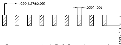
Recommended P.C.Board Layout
